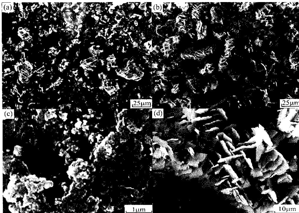
Fig. 6. SEM micrographs of phase extracted precipitates after filtering. (a) Tensile tested at 760°C (b) Tensile tested at 816°C (c) High magnification of (a) (d) High magnification of (b)
