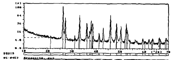
Fig. 1. XRD analysis of sepiae os. Standard material used was CaCO 3 .
