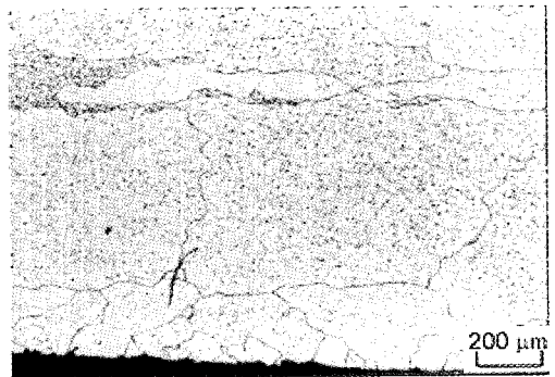
Fig. 3 Optical micrograph of a sample with large grains. The sample with this type of microstructure was designated as type 'B'
