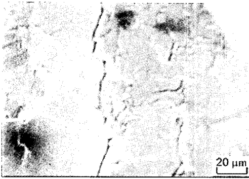
Fig. 11 SEM micrograph of the fractured surface after fatigue test. The liquation crack was observed
