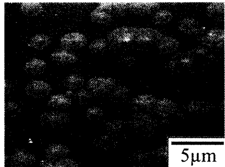
Fig. 2. SEM image of PLZT thin film annealed at 650°C for 30 min.
