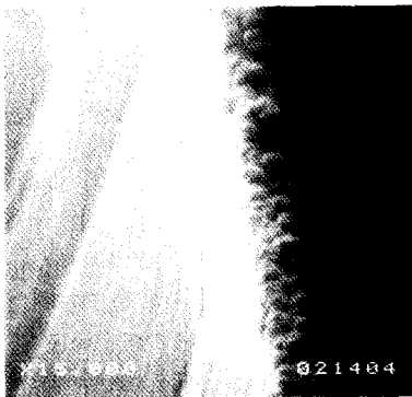
Fig. 5. SEM photographs of the cross section for the \text{BaTiO}_3 thin films annealed at 800°C.
