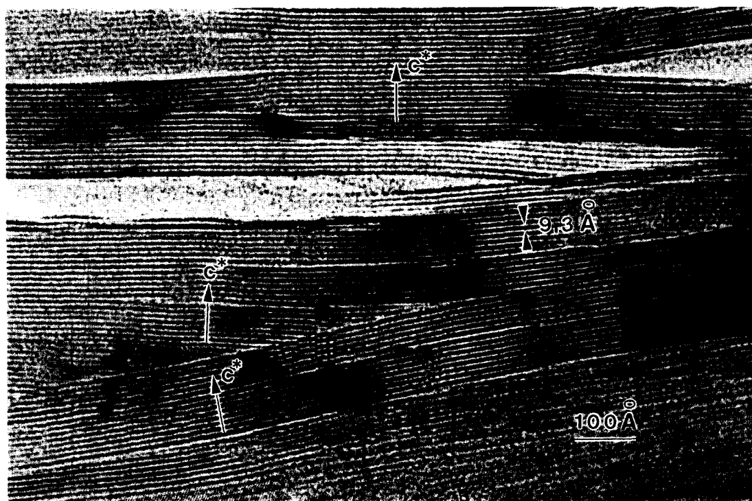
Fig. 4. HRTEM image of talc composed of subparallel packets of talc layers. Packets of talc layers intersect subparallel layers at the boundaries, resulting in low-angle grain boundaries.
