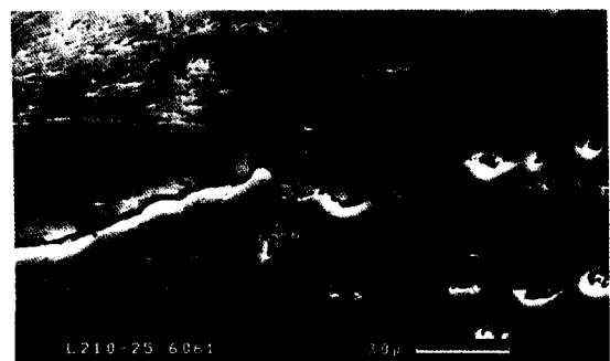
Fig. 3 Typical HAZ grain boundary liquation cracking in the laser welded 6061 alloy.
