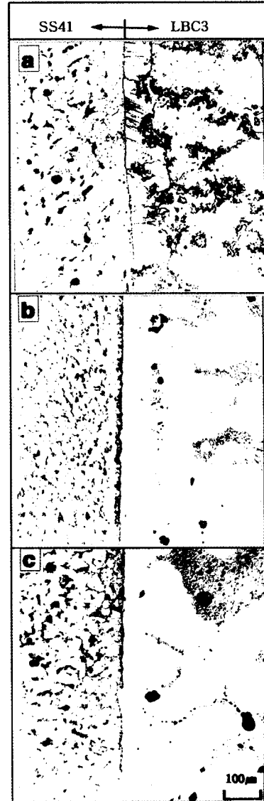
Fig. 5 Optical micrographs of interface of the bonded SS41/LBC3 at 850℃ for (a) 10 minutes, (b) 30 minutes and 60 minutes
