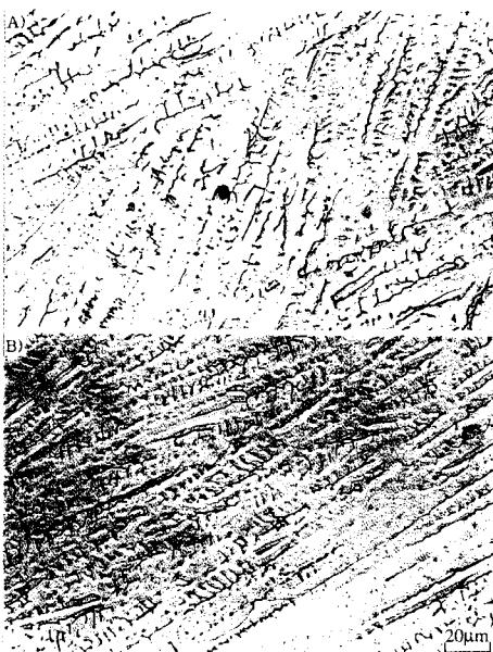
**Fig. 4** Microstructures of GTA welds, mixed acid.
