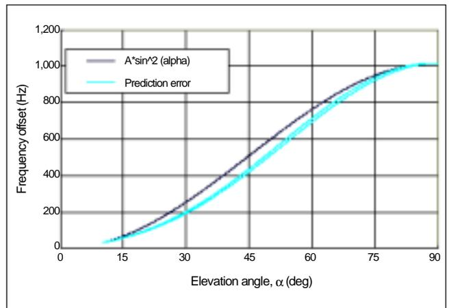
Fig. 5. Prediction error of doppler frequency shift versus the satellite elevation angle.
