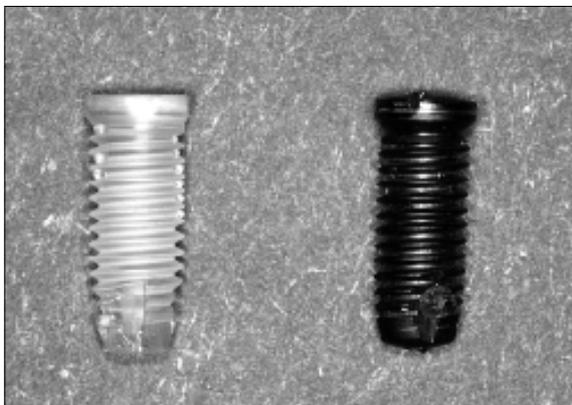
Fig. 1. Photograph of epoxy resin implant replica and titanium coated epoxy resin implant. The coating thickness is 1000-1500 Å.
