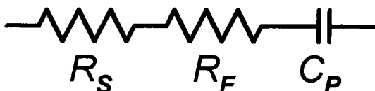
Fig. 2. The simplified interfacial equivalent circuit for the intermediate frequencies.
