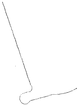
Fig. 18 Shape of the keel in the energy storing prosthetic foot obtained from the external work minimization
