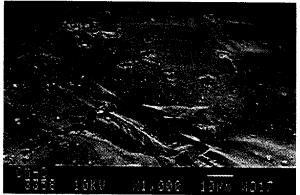
(b) Contact mass before reaction (composition: Cu/Si = 7 wt %, Zn/Cu = 15 wt %)
