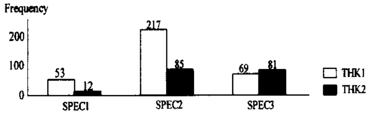
두께 : THK1 2.3~4.5mm, THK2 4.5~8.5mm 탄소함유량 : spec 1 0.02~0.06%, spec 2 0.05~0.08%, spec 3 0.16~0.20%
