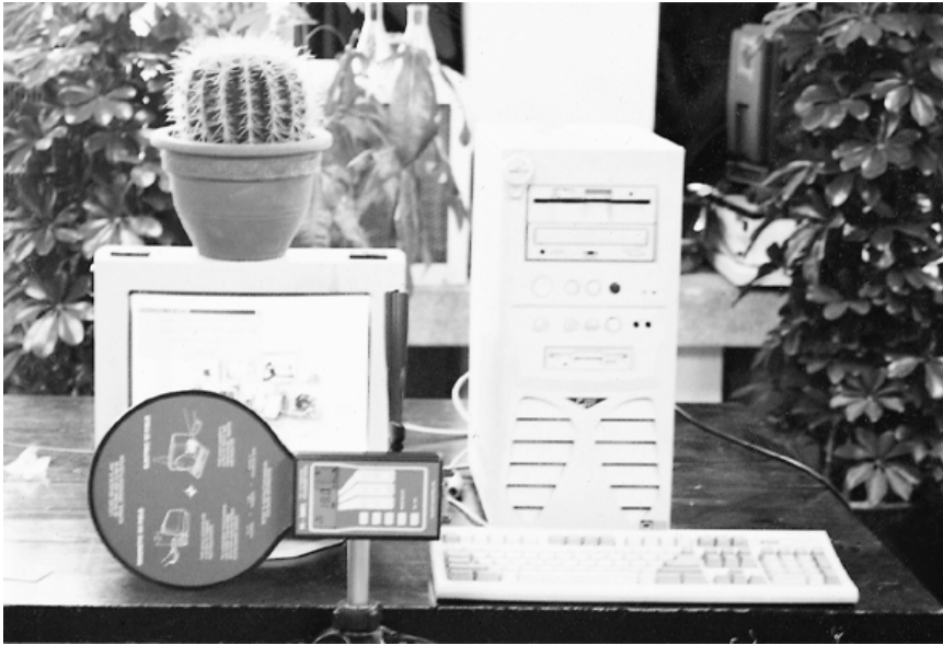
Fig. 1. Apparatus for measuring electromagnetic waves (ELF and VLF) and computer monitor used in this experiment.
