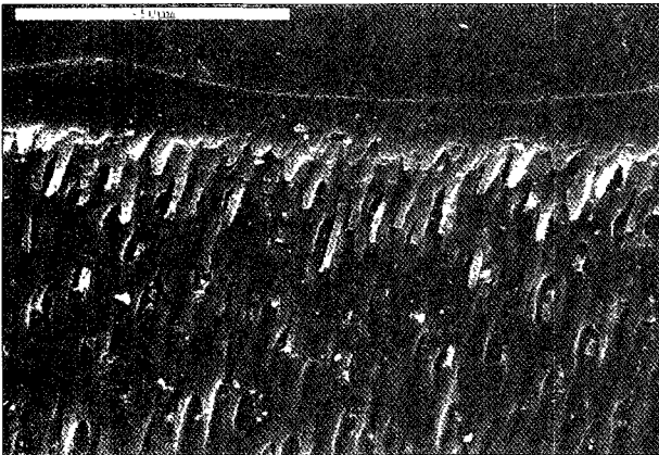
Fig. 5. Hybrid layer, adhesive layer and resin tags of the specimen bonded with Single Bond Dentin bonding system (magnification \times 1000 )
