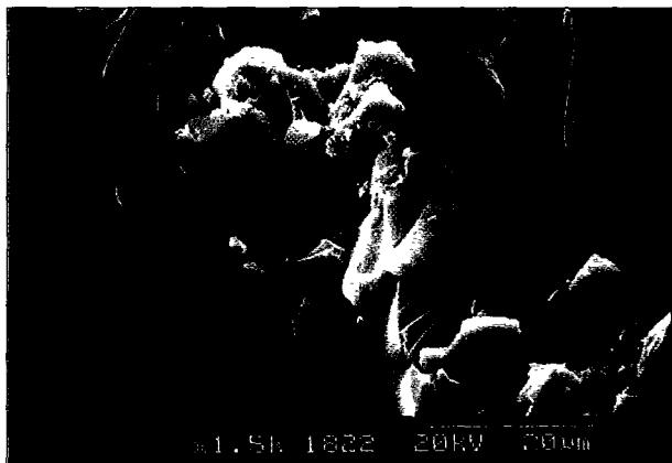
Fig. 5. Fracture surface of crushed silica group. Cut surface of resin matrix and the interface between resin and filler is obvious ( $\times 1500$ ).
