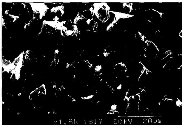
Fig. 1. Powders of crushed silica( $\times 1500$ ).
