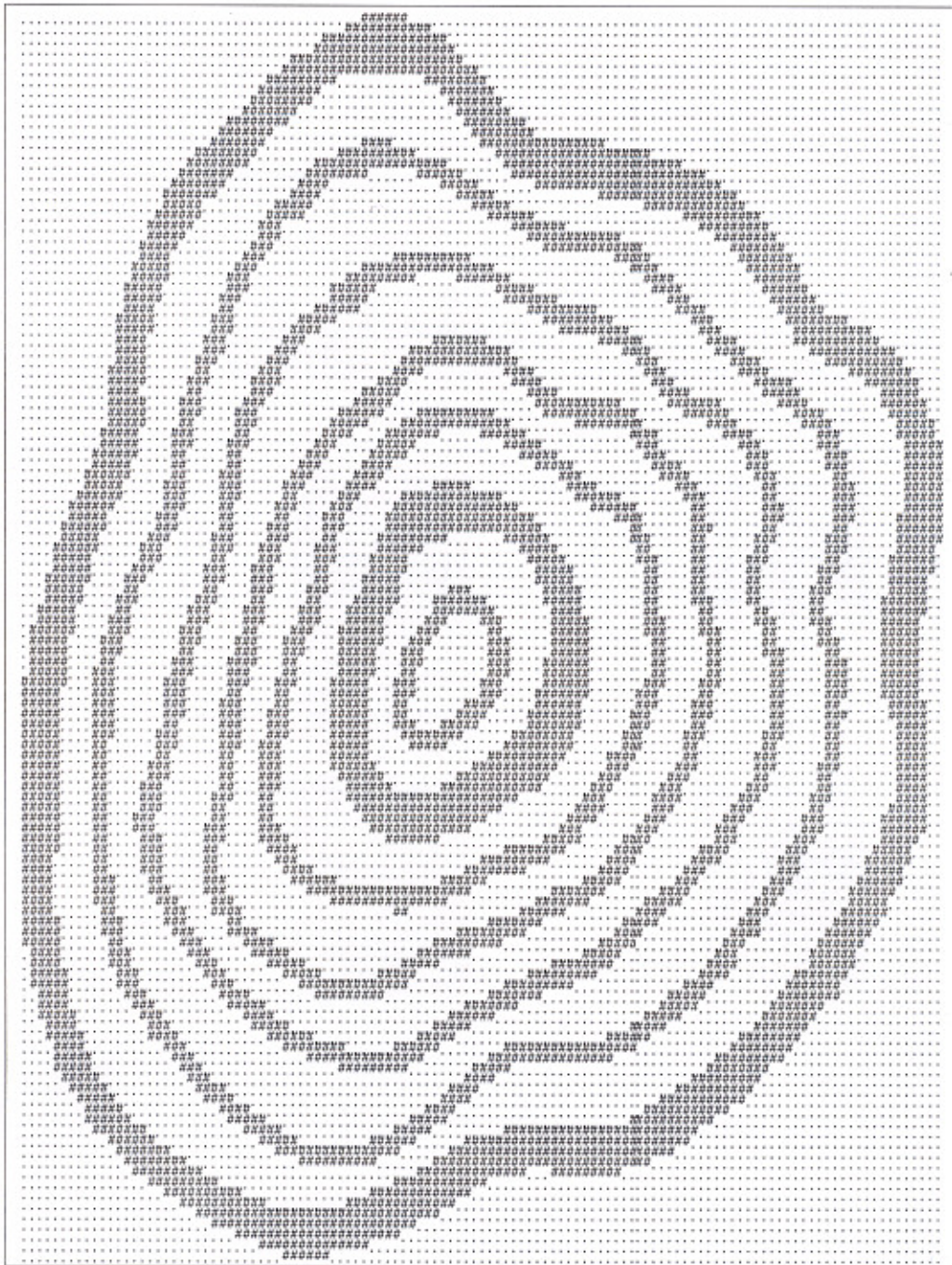
FIGURE 7. Converted picture as '.' and '#' for each pixel in the Fig. 6
