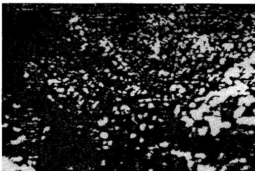
Fig. 3. Surface morphology of EVA/carbon black (50phr) composite from solution process.
