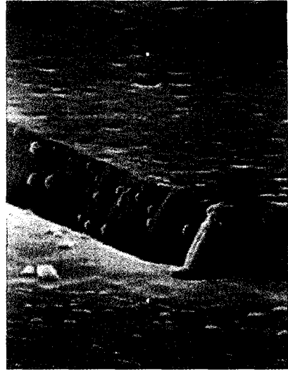
Fig. 5. SEM micrographs of PR masked GaN etched by 60%Cl 2 /40%HBr plasma
