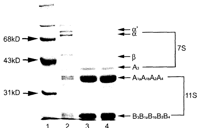
Fig. 1. SDS-PAGE electrophoresis of 11S glycinin purification. Lane 1: Molecular weight marker. Lane 2: Defatted soy flour extract. Lane 3: pH 6.4, precipitated 11S rich fraction. Lane 4: 11S glycinin eluted from affinity chromatography. \alpha , \alpha' , and \beta are identified as 7S conglycinin. A and B indicate the acidic and basic subunits of 11S glycinin, respectively.
