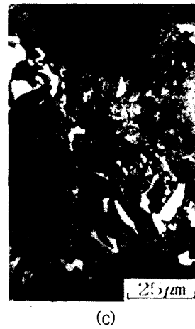
Photo. 3 Optical microstructures of ductile iron coated with black paint and laser surface hardened for output power of 1600w at a given traverse speed of 2.0m/min. (a) Hardened zone, (b) Heat affected zone, (c) Matrix
