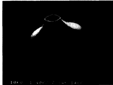
(a) 원모양 범프(등방성 식각) (a) circular bump(isotropic etching)
