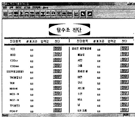
Fig. 9. Diagnostic window of dewatering tank.
