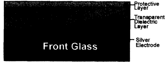
Fig. 1. Schematic diagram of fabricated panel structure.
