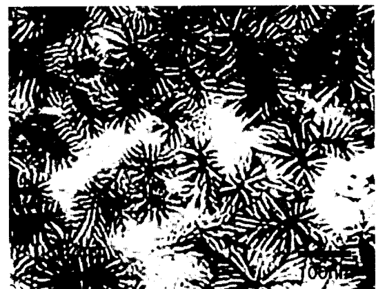
Fig. 1. Corresponding microstructure of Co-22%Cr films at the substrate temperature of (a) room temperature and (b) 200°C
