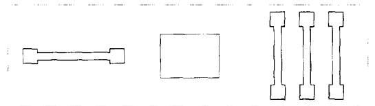
Fig. 2. The shape of shadow mask used to make the tunneling junctions. Each layer is grown successively.
