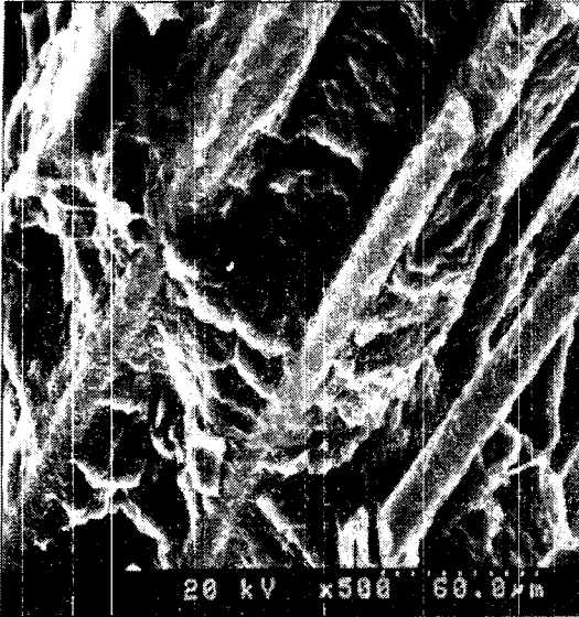
Fig. 8. SEM photograph of impact fracture surface for various fiber fraction GF/PP tested at room temperature.
