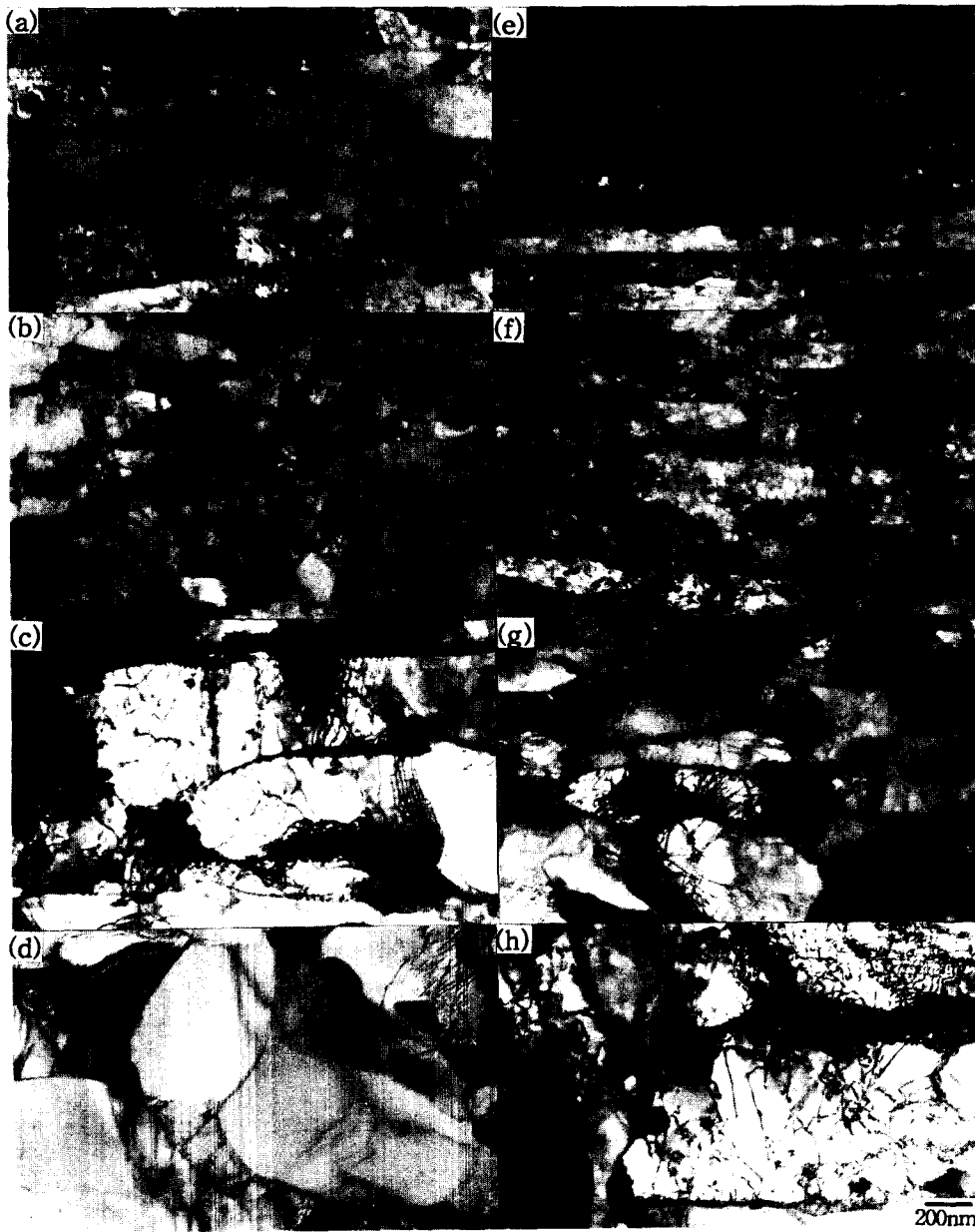
Photo 1. Tempered martensite structure of Mod.9Cr-1Mo steel (a-d) and 9Cr-0.5Mo-2W(e-h) steel : tempered at (a,e) 650°C (b,f) 700°C (c,g) 750°C (d,h) 800°C
