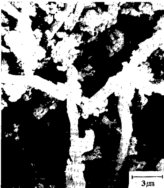
Fig. 2. Scanning electron micrograph of alumina hydrate-coated SiC whiskers, [Al_2(SO_4)_3] : 0.025 mol/l, [SiC] : 9.0 g/l and ageing time: 100 h.
