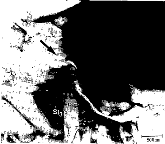
Fig. 8. Example of TEM micrograph for crack propagation (denoted by arrow) along grain boundary of coarse acicular \text{Si}_3\text{N}_4 grain.
