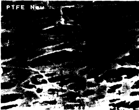
Fig. 6. SEM micrograph of new PTFE membrane surface.
