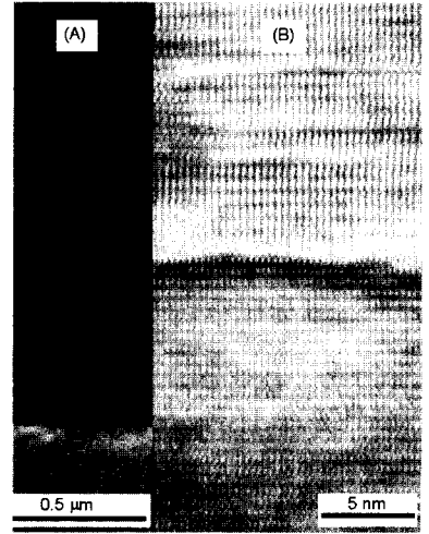
Fig. 4. (a) Bright field and (b) high resolution TEM image of interface of GaN/sapphire thin films with [1120] zone axis.
