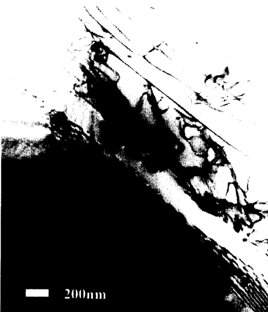
Fig. 3. TEM image of dislocations concentrated near microdomains in the MgO doped LiNbO 3 .
