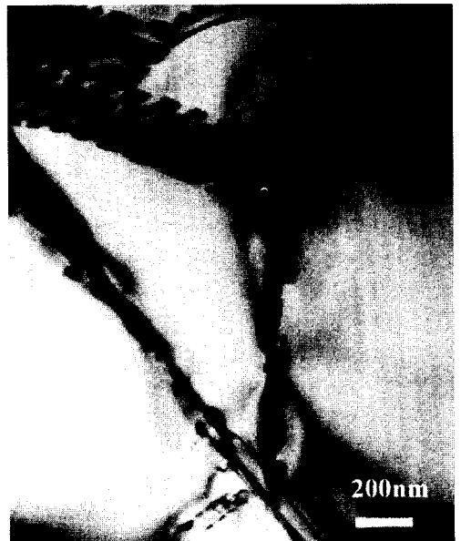
Fig. 2. TEM image of microdomains trapped by defects.
