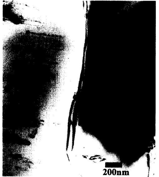
Fig. 4. Subgrain boundary formed by align
