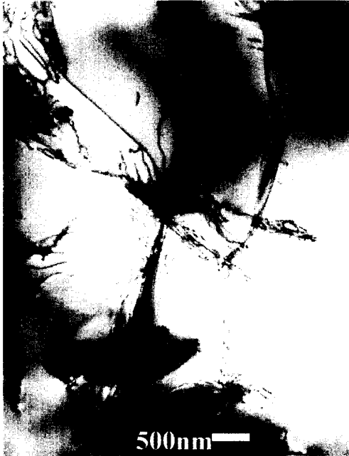
Fig. 8. TEM image of defects concentrated in the tail.
