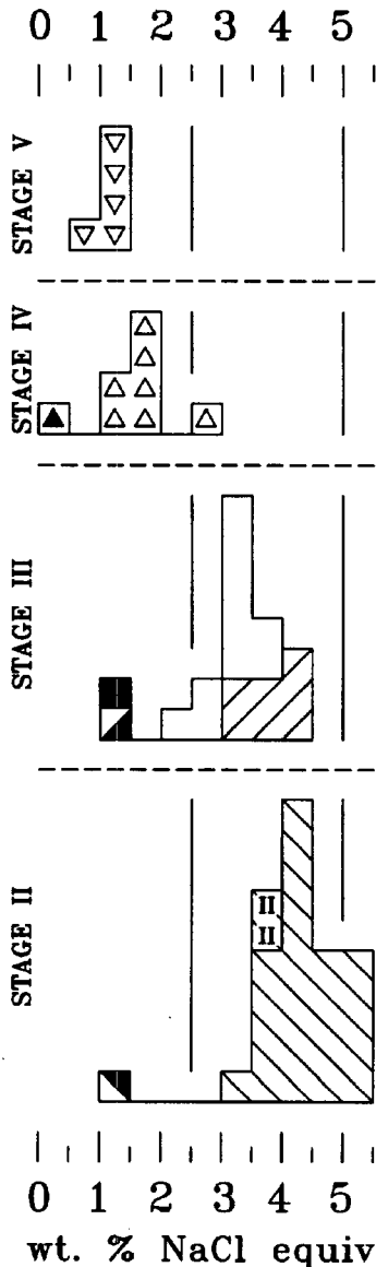
Fig. 6. Frequency diagrams of salinities of fluid inclusions in vein minerals from the Hyundong antimony deposits. There is a general decrease of salinity with elapsed time. Symbols are the same as in Fig. 5.
