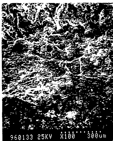
Photo 3. SEM photograph of 2L bending fatigue specimens
