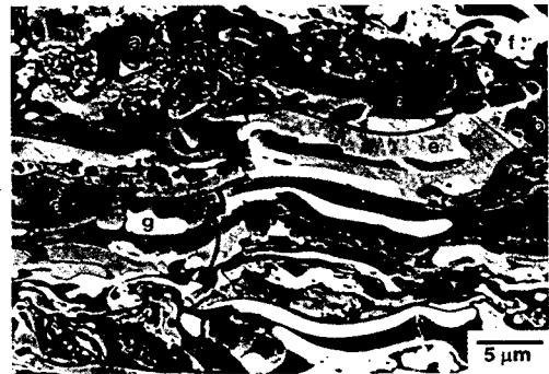
Fig. 4 Back scattered electron image of plasma-sprayed WC-12%Co coating.
