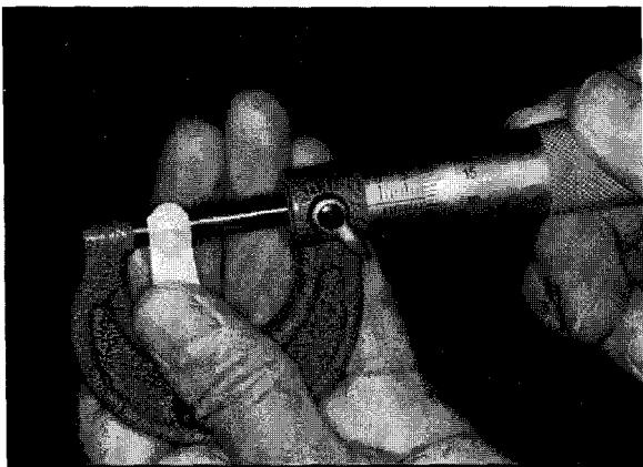
Fig. 2. The use of a micrometer to obtain standard measurements.
