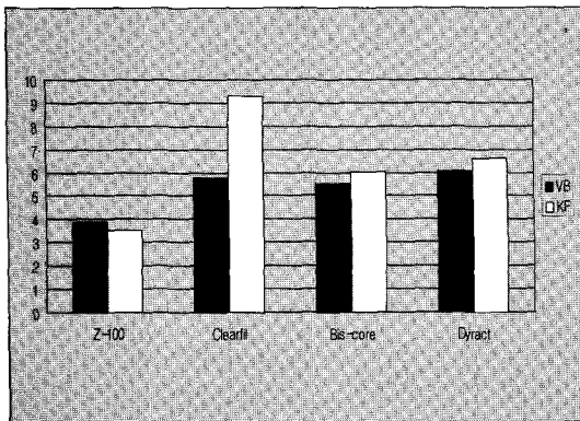
Fig. 4. Comparison of shear bond strengths of 4 composite resins to 2 GIC bases, MPa, n=10
