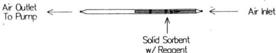
그림 1. Standard glass detector tube filled with a solid sorbent coated with a chemical reagent.
