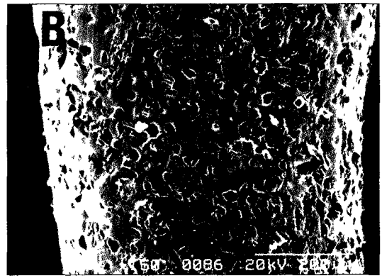
Fig. 1. Scanning electron micrograph of surfaces of ultrasonic instruments (original magnification X150). A, a stainless steel instrument showing a smooth surface. B, a diamond instrument showing a rough surface with diamond particles.
