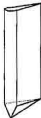
(a) A shape of triangular chisel
