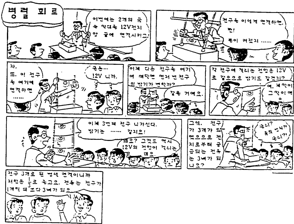
Fig. 2 The textbook explanation about the brightness of bulbs connected in parallel
