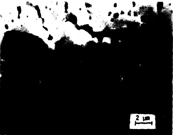
Fig. 9. Cross-sectional BEI of the oxidation products in the thermally cycled EB-PVD TBC.
