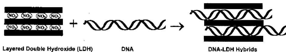
Fig. 16. Schematic diagram for DNA encapsulated with LDH.
