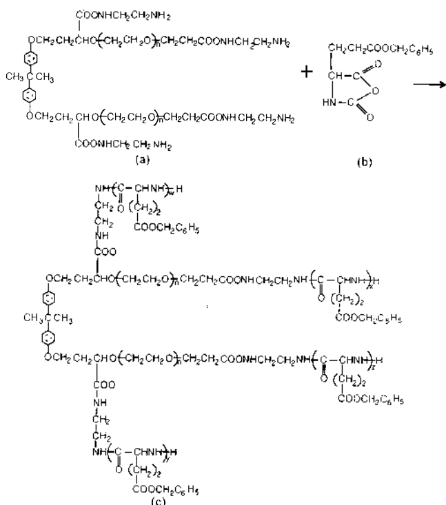
Figure 1. Synthesis scheme of PBLG/PEO/PBLG (GEG) block copolymer: Bis[poly(ethylene oxide)bis(amine)] (a), \gamma -benzyl L-glutamate N-carboxyanhydride (b) and GEG block copolymer (c).
