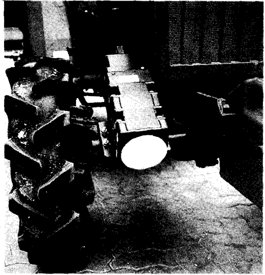
Fig. 3 A radar speed sensor installed at the front of tractor.
