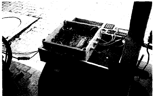
Fig. 4 A control console consisting of a datalogger and relay drivers.
