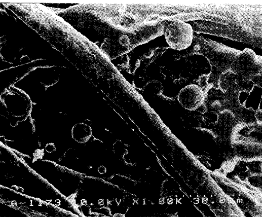
Fig. 12 SEM photographs of cotton fabrics treated with poly(L-lactide) microcapsules after laundry tests ; control (upper), 10 times (middle), 15times (lower).
