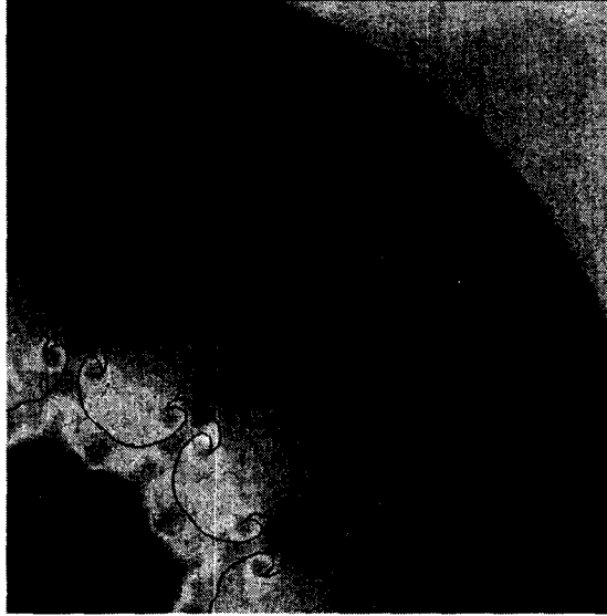
FIGURE 5. The simulation of Richtmyer-Meshkov (RM) instability in the cylindrical coordinate. The dense black line represents a tracked interface and it conserves the symmetries of the mushroom shape of growing interfaces.
